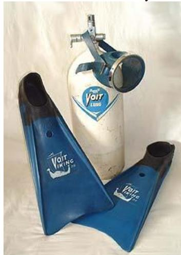
**Tanks** - cylinders should be rinsed in fresh water after use and then wiped dry. Remove the tank boot so that no water accumulates and starts to rust the tank. Crack the valve briefly to blow out any moisture from the valve opening.
