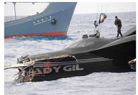
Last year, the *Ady Gil* was cut in half after a collision with the *Nisshin Maru* a Japanese security ship. The \$1.5 million dollar carbon fiber and Kevlar ship sank shortly thereafter.
